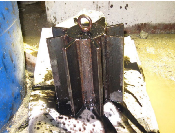
A heavy plumb bob with fins (left) and submerged in a container of oil during the observation (right).
